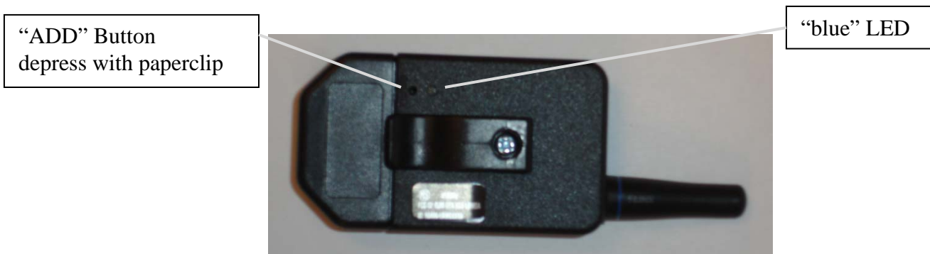
Fig. 1: Keyfob Back Button Assignments
