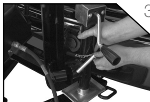
3. Remove crankstand from lift frame.
