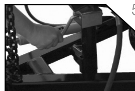
5. Adjust crankstand until crankstand comes into contact with the ground and then turn 1 to 2 revolutions.
