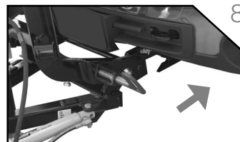
8. Back vehicle away from plow assembly.
