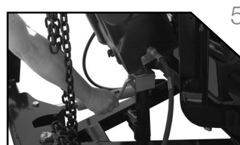
5. Adjust crankstand until crankstand comes into contact with the ground, then turn 1 to 2 revolutions.
