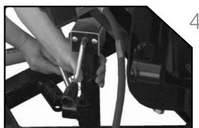
4. Attach crankstand to a-frame..
