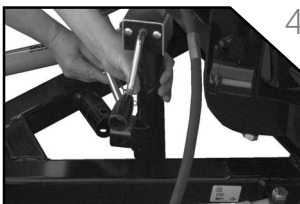
4. Attach crankstand to A-frame.
