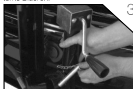
3. Remove crankstand from lift frame.
