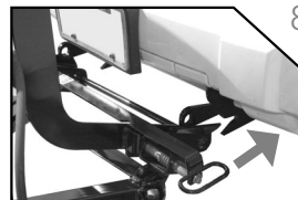
8. Back vehicle away from plow assembly.
