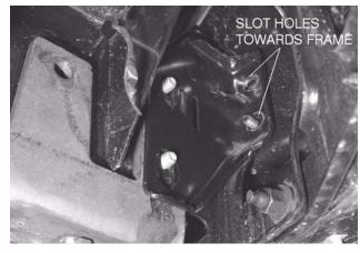
D. Attach Universal Clevis (\*) between Hanger Weldments (2&3) using four 1/2-13 x 1 3/4" bolts (8), and 1/2-13 locknuts (12) on each side. Lower holes on Hanger Weldments (2 & 3) may need to be used due to vehicle configuration. Note: Bumper may need to be notched around front lobes of Universal Clevis (\*).
