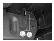
The upper holes (A) must be drilled. Using the L.H. & R.H. Side Mounts (1 & 2) as a template drill 2 holes 9/16" diameter thru the vehicle frame and fasten using Bolt H 1/2-13 x 5-1/2" (10), 1/2" Flatwasher (11) and 1/2-13 Locknut (8). On bottom holes use the original tow hook fasteners.
