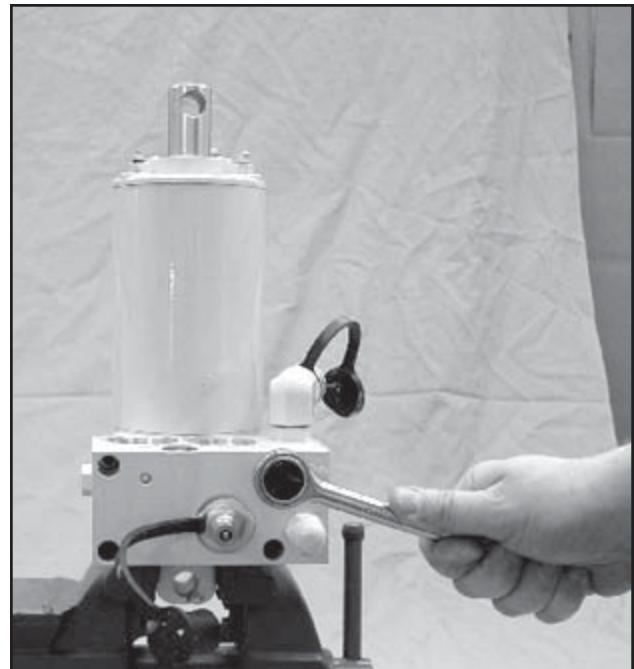
FIGURE 3-21 The valve body can be removed from unit using a 1/4" hex key or Allen Socket.
