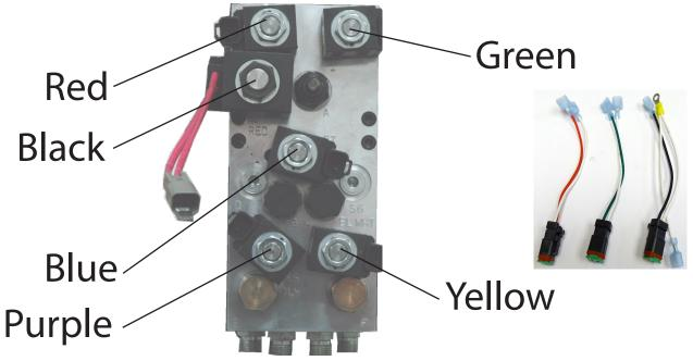
Step 5: Connect the six coil adapters (7) (red, green, black, blue, purple and yellow) to the Harness (4) (brown to white, red to red, black to black, green to green, blue to blue, purple to purple and yellow to yellow). Connect the heavy black wire to the motor ground as shown (A). If motor does not have a ground lug connect heavy black wire to the Hydraulic Block.
