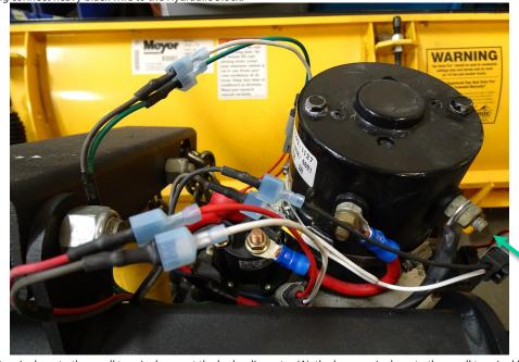
Step 6: Connect White wire loop to the small terminal nearest the hydraulic motor (A), the brown wire loop to the small terminal farthest from the hydraulic motor (B). Connect the heavy red wire to the large terminal of the motor solenoid (C).
