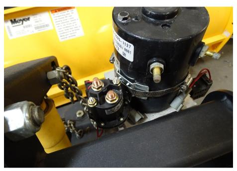
Step 3: Attach SOS Motor Cable (5) from the Motor Solenoid (2) to the hydraulic unit motor as shown.
