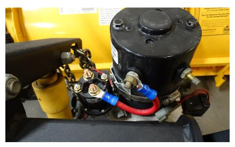
Step 4: Connect the three coil adapters (7) (red, green and black) to their respective coils.
