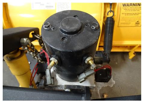
Step 2: Clamp on Motor Solenoid (2) using Clamp (1) to the hydraulic unit.
