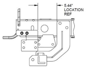
Note: Before tightening the fasteners, the Clevis Frame (\*) should be level with the ground and pushed back as far under the vehicle as possible.
