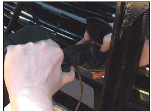
G. Disconnect one piece electrical plug and install weather cover on male end.
