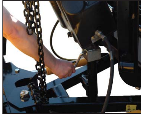
E. Adjust crankstand until crankstand comes into contact with the ground and then turn 1 to 2 revolutions.
