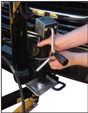
B. Push lift arm down until there is slack in the chain.
