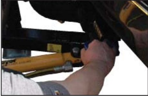
B. Twist handles on both sides to engage spring loaded pins.
