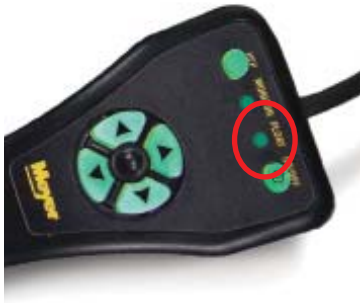
A. Press down button until float light turns blue.
