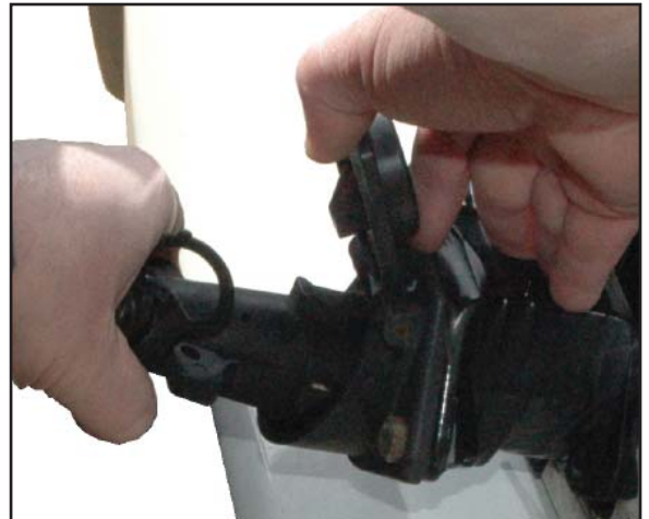
G. Remove weather cover on male end and connect one piece electrical plug. The spring loaded cover will lock one piece plug.
