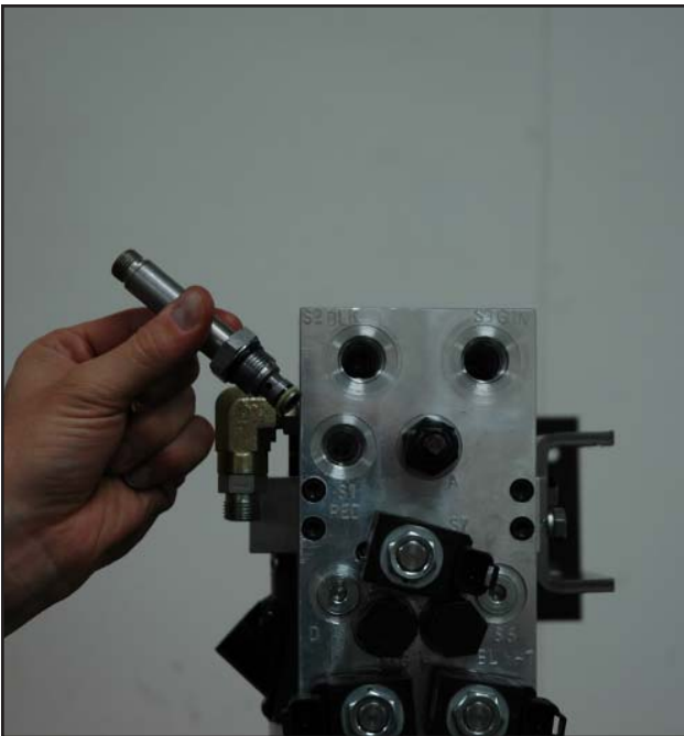
FIGURE 3-12 The "S1" Cartridge is removed. Clean by soaking cartridge in cleaning solvent.
