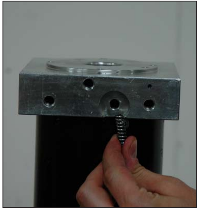
FIGURE 3-59 Remove pump pressure adjustment spring.
