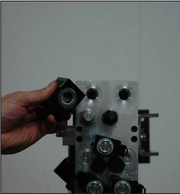
FIGURE 3-10 Coil removed from the "S1" Cartridge.
