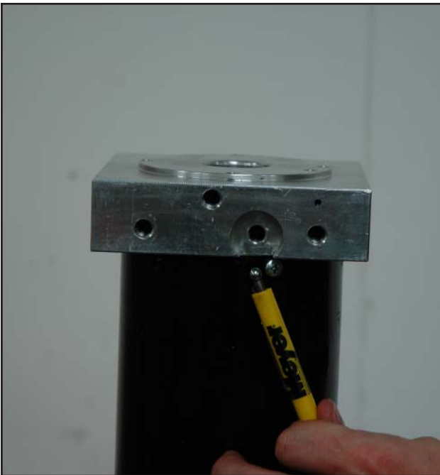
FIGURE 3-60 Remove pump pressure adjustment ball.
