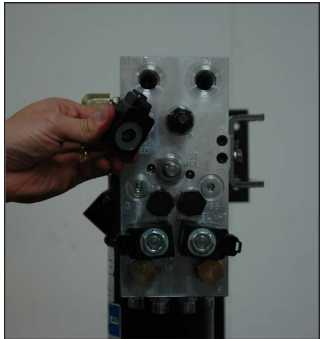
FIGURE 3-13 Coil removed from the "S7" Cartridge.
