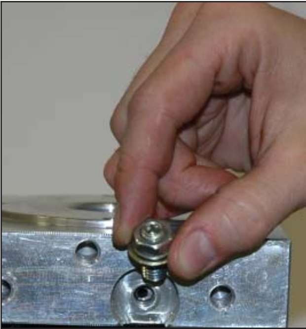
FIGURE 3-58 Remove pump pressure adjustment assembly.
