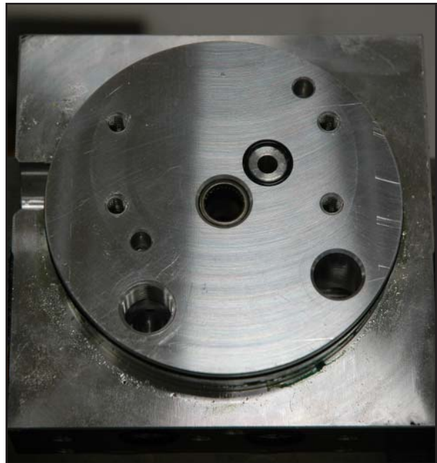
FIGURE 3-61 Inspect base and clean base in cleaning solvent.
