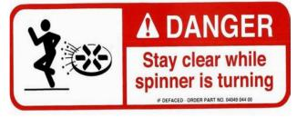
This decal appears on the back of the spreader trough cover plate. It alerts all to the danger of being caught in the dropout opening or from the top of the spreader trough where serious personal injury could result.
