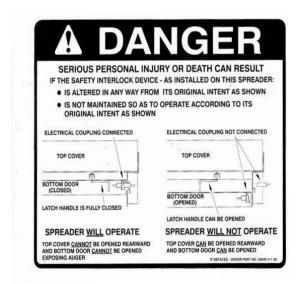
This decal appears on the back of the spreader cover plate at the right end of the spreader. It alerts all to the danger associated with the improper use of the Safety Interlock Device.
