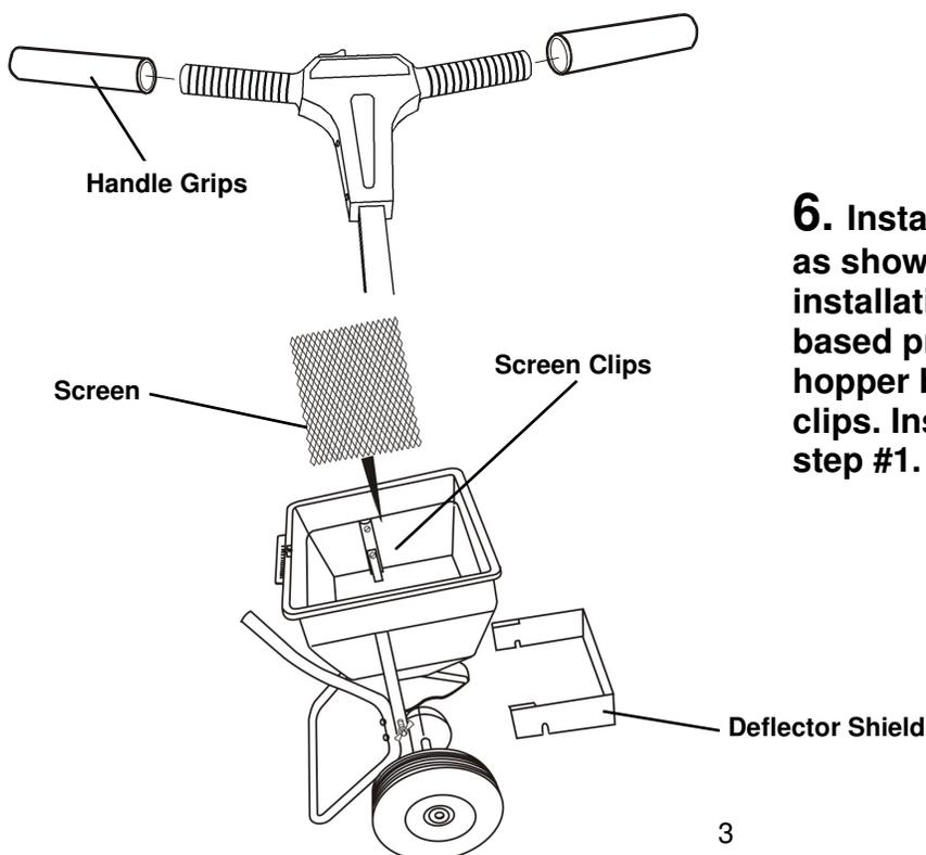
**6. Install handle grips onto the handle as shown. Soapy water will ease installation. (Do not use petroleum based products). Insert screen into hopper by sliding it under the screen clips. Install deflector shield removed in step #1.**
