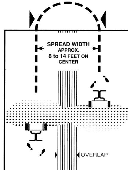
**7.** Push spreader 2 1/2 m.p.h. (18 feet in 5 seconds) for full 8' to 14' spread pattern when applying fertilizer products. Apply header strips at each end of area to be treated then space trips across the area as shown.
