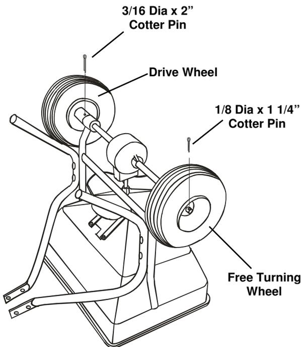
**2.** Slide wheels onto end of axle with the hub facing toward frame. Wheels are identical to ease assembly. Align the hole in the wheel hub and the hole in the axle as shown. Secure drive wheel to axle with 3/16 dia x 2" cotter pin. Insert 1/8 dia x 1 1/4" cotter pin in the hole near the end of axle to retain free turning wheel.
