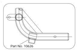
Attach underframe (2) at the outer two holes, in crossmember, using 1/2-13 x 2" bolts (11), flatwashers (13), and locknut (15), and at the center hole using handle bolt (4), flatwasher (14), and locknut (16).
