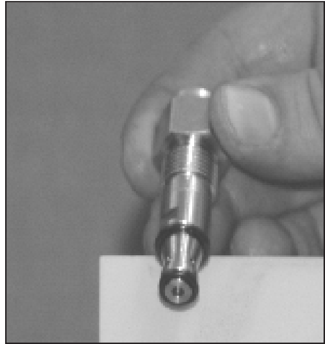
FIGURE 3-108 Insert small O-ring into the Crossover cavity of the P.A. Block. Make sure small O-ring fits flat in the bottom of the cavity.
