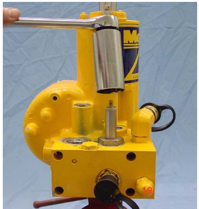
FIGURE 3-29 Remove "C" Cartridge using a 1-1/4" hex head deep well socket.
