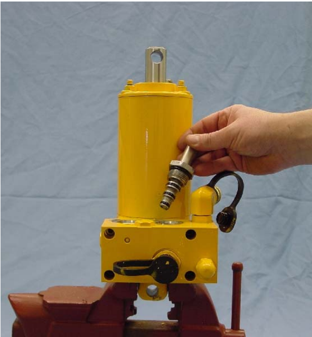
FIGURE 3-30 Remove "C" Cartridge from Sump Base.
