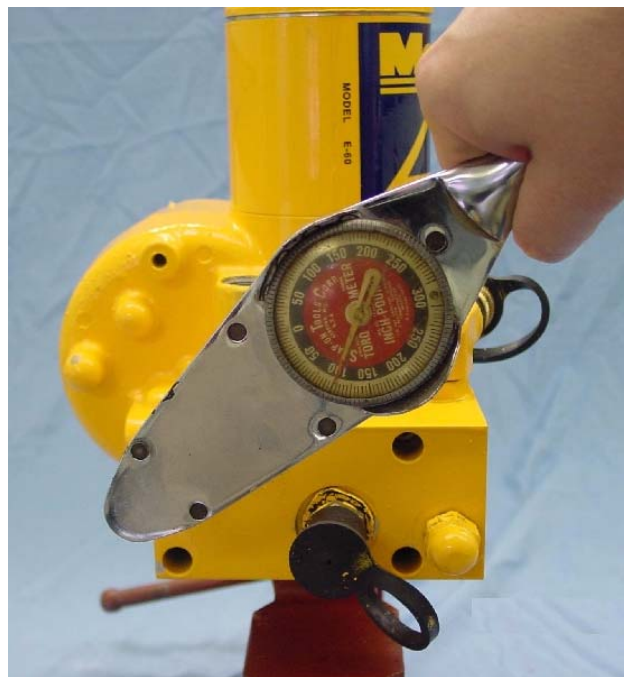
FIGURE 3-71 Install P.A. Block Assembly using 5/16-18 x 1-1/2" soc. head screws. Torque to 96-120 in. lbs.
