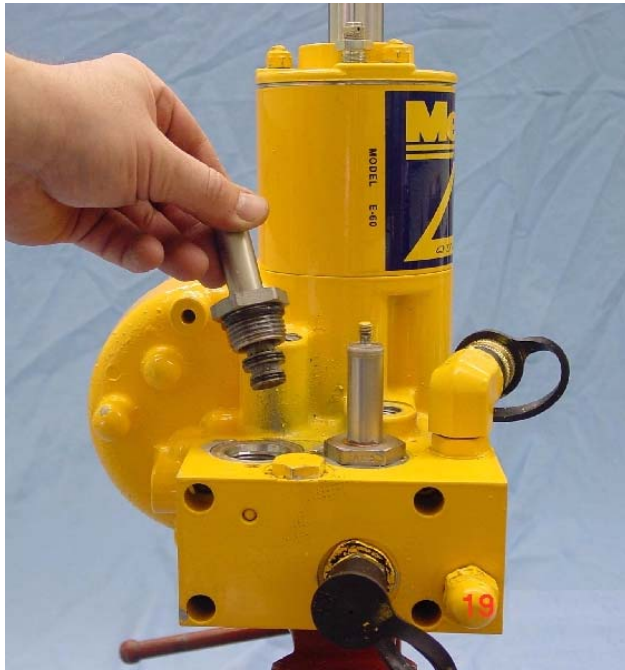
FIGURE 3-26 Remove "B" Cartridge from Sump Base.
