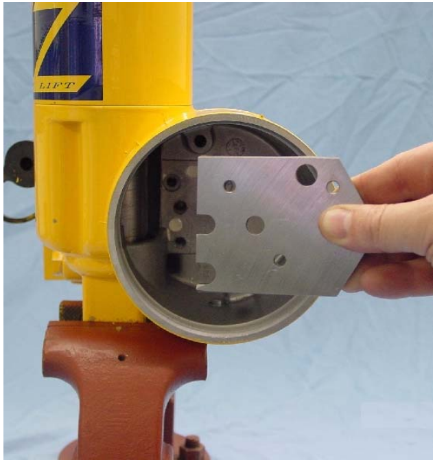
FIGURE 3-10 Remove Pump Mounting Plate.
