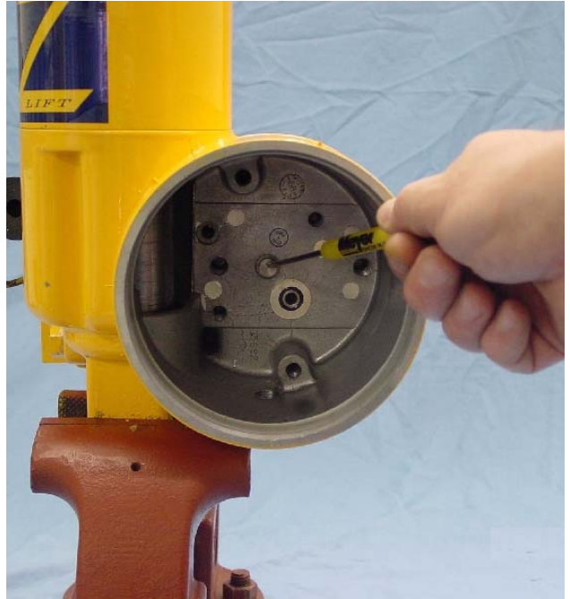
FIGURE 3-11 Remove Pump Mounting Plate Locator Pin.
