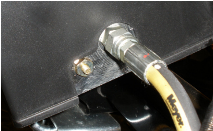
E-58H Lower Adjustment (left side of vehicle): Loosen jam nut and turn screw clockwise to slow the drop of the plow and counter clockwise to speed the drop of the plow. Tighten jam nut.
